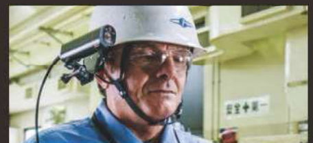
The camera-head can be attached to a helmet with a sense of wearable or the controller, and can be attached to a pole as camera stick.
